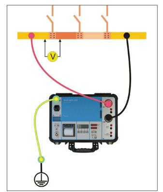
Using an external voltmeter, measure the voltage drop (voltage) across each contact element within every section of the bus-bar being tested.
