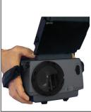
Superb-OD & Superb-XD are portable handheld daytime corona and arcing recording cameras. Superb models are robust solar blind bi-
