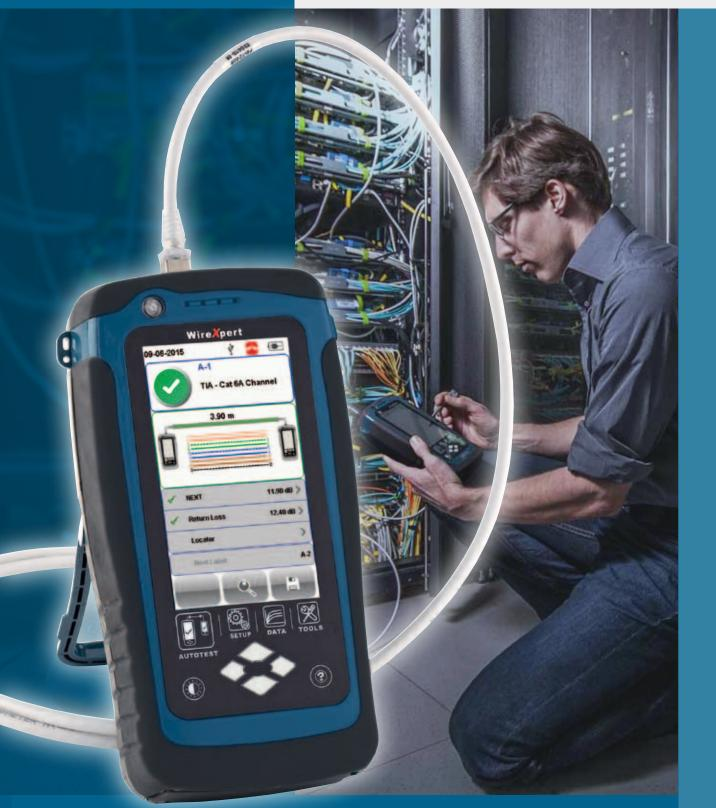
WireXpert 500 is the most affordable copper cable certification tester for twisted pair cabling systems with performance levels up to CAT6A/Class  $E_A$ . Electricians and network cabling contractors can perform certification testing on copper installations with speed and accuracy using WireXpert 500. In addition to standards based permanent link and channel certification, WireXpert 500 offers optional test adapters for coaxial cable testing and patchcord testing.
